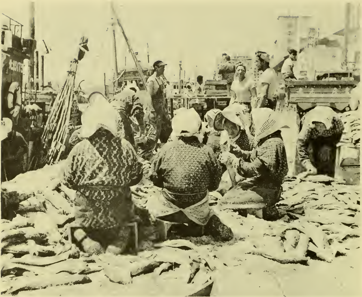
Figure 5. --Women sorting salted salmon by species, removing excess salt and segregating damaged fish.
