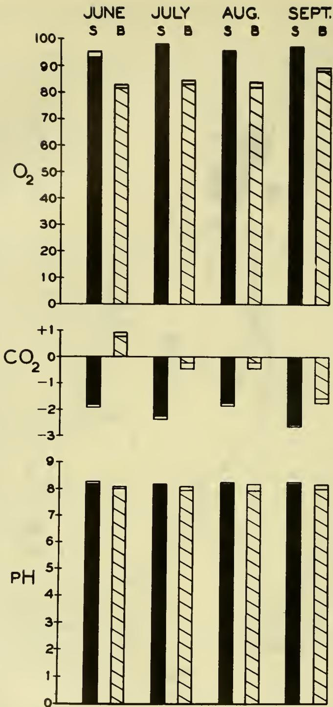
Figure 37. --The means and probable errors ( $r_o$ ) of the oxygen saturation, carbon dioxide, and hydrogen-ion determinations on the surface and bottom waters of Lake Erie, 1929.
