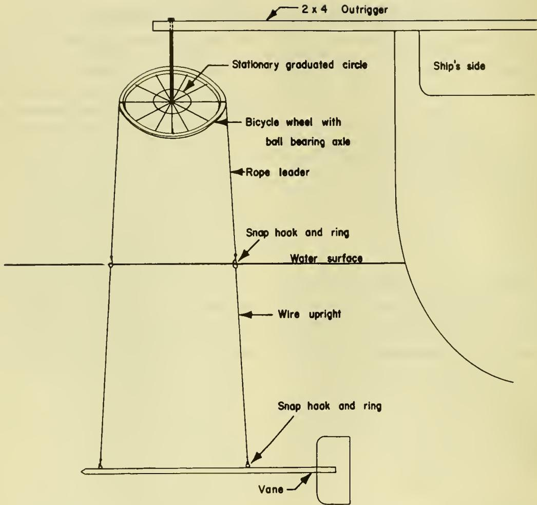
Figure 3. --Subsurface current-direction indicator.
