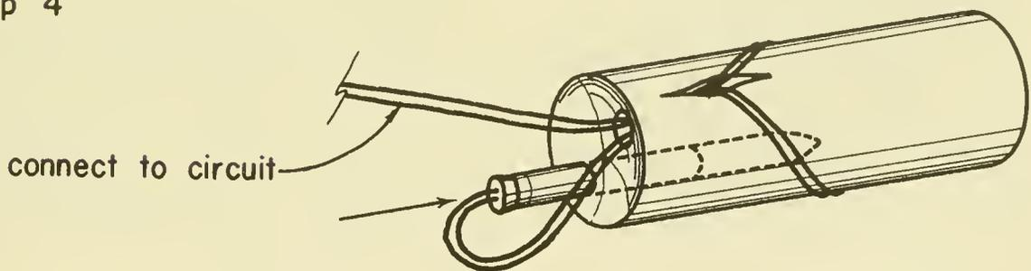
Figure 5.--Method of capping dynamite.
