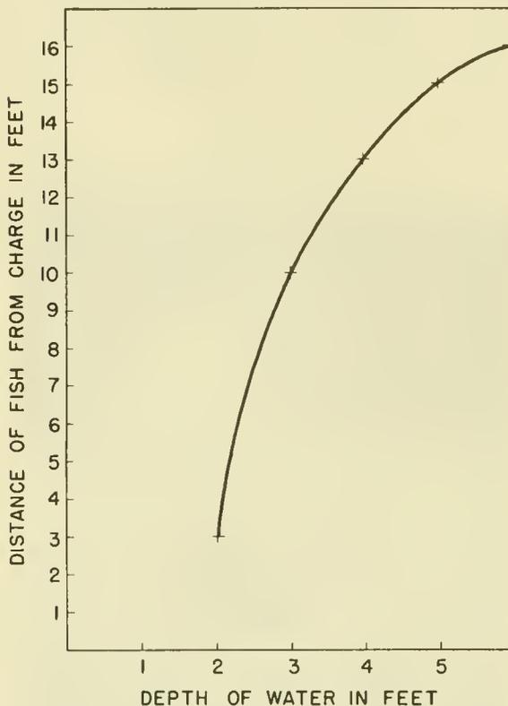
Figure 2.--Lethal range of one-half stick of dynamite in water of various depths.
