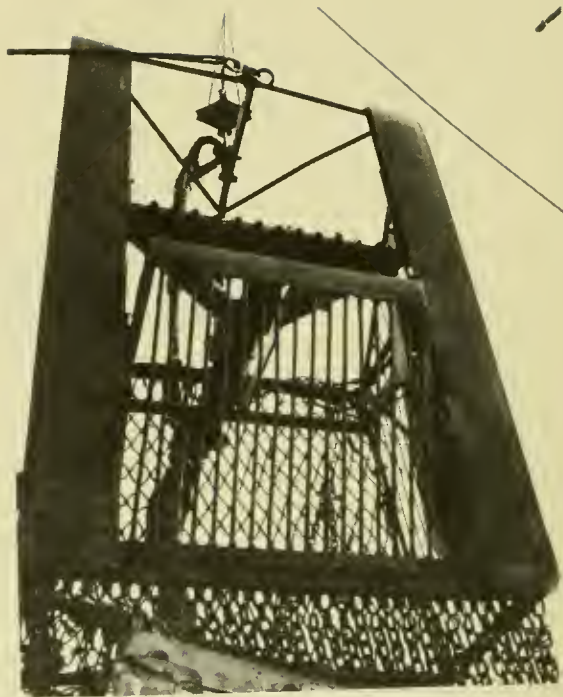
Figure 1. Bottom view of the forward cage of a jet dredge
