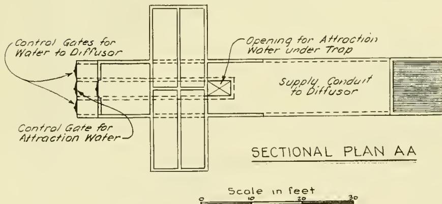
Figure 3:--Design drawings of upstream trapping system including trap and holding pens. The water path through the holding pens and trap is indicated.
