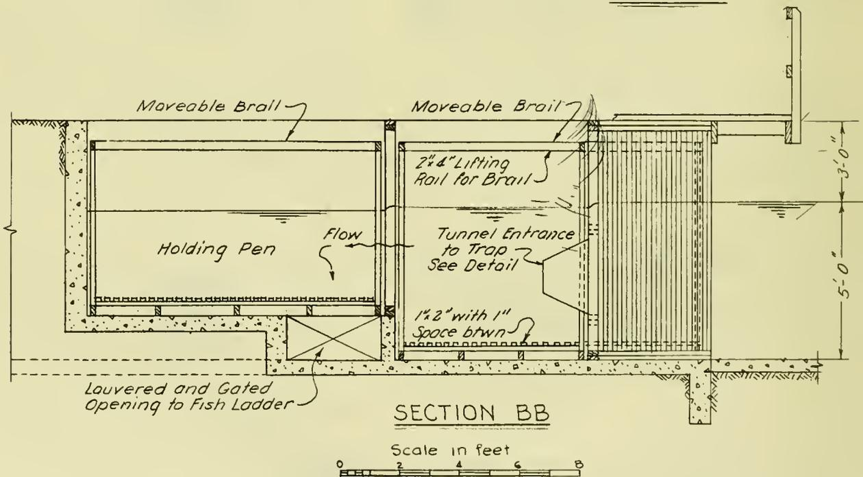
Figure 4:--Design drawings of downstream trapping system including trap and holding pen. Details of the tunnel entrance and flow pattern are shown.
