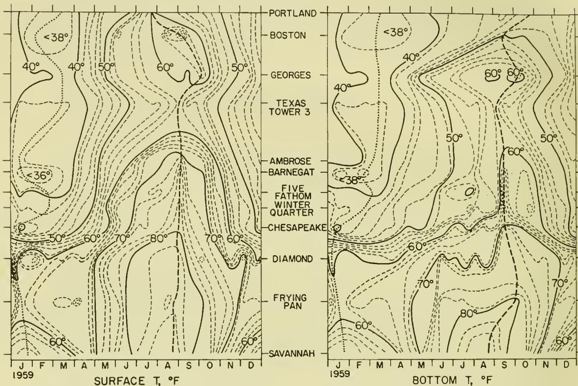
Figure 1. The cycle of temperature at the surface (left) and bottom (right) along the series of observation posts for 1959. Heavy dotted and dashed lines indicate minimum and maximum temperatures respectively.
