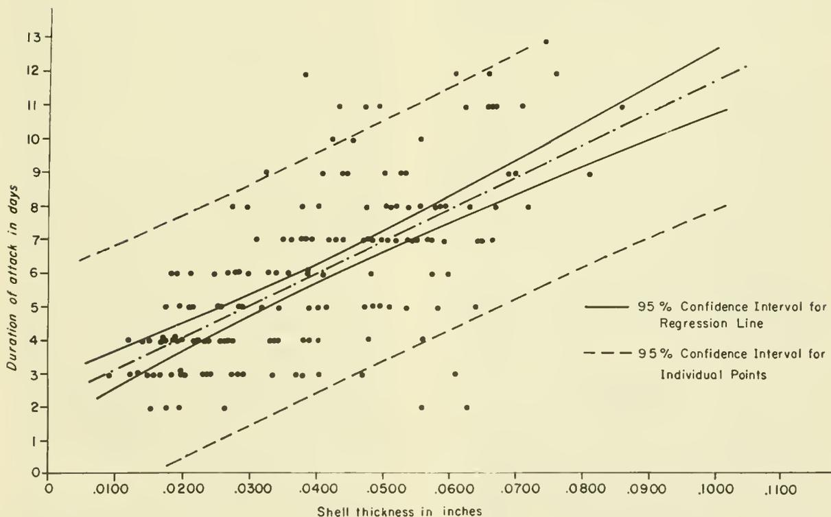
Figure 6.--Regression line and scatter diagram of duration of attack upon thickness of all shells from Experiment I.
