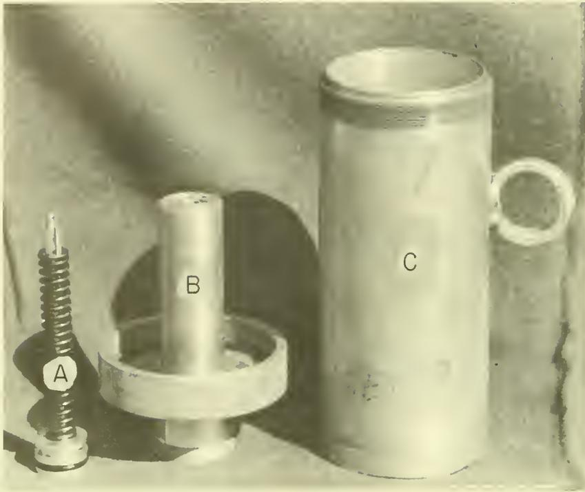
Figure 1.--Three assembly groups for the bathykymograph. A - the pressure sensing piston assembly, B - the piston housing, and C - the case.
