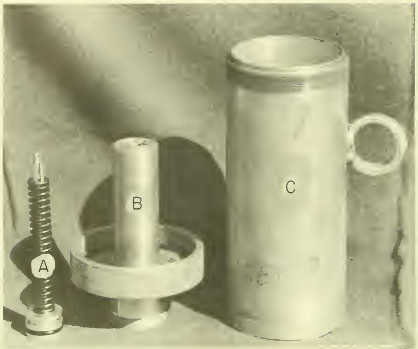
Figure 1.--Three assembly groups for the bathykymograph. A - the pressure sensing piston assembly, B - the piston housing, and C - the case.
