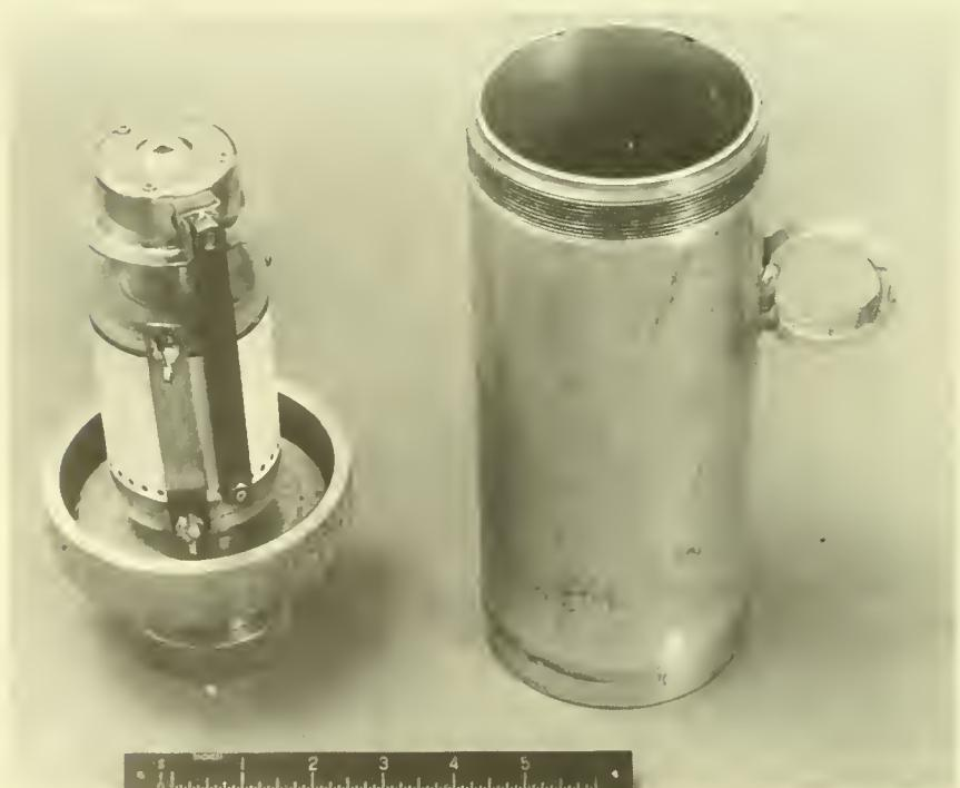
Figure 2.--Assembled bathykymograph with cover removed.
