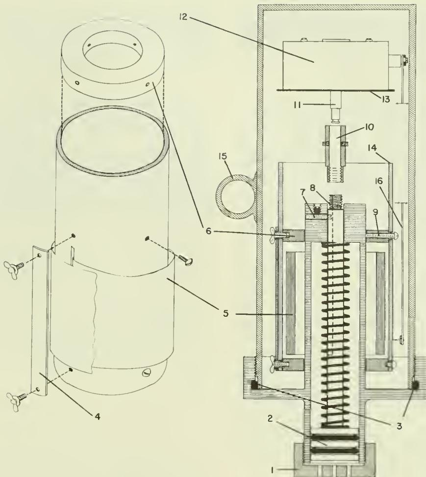
Figure 3.--Sectional view of bathykymograph. See text for explanation.
