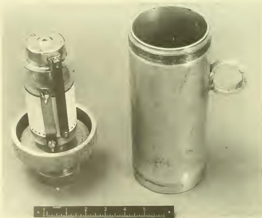
Figure 2.-- Assembled bathykymograph with cover removed.
