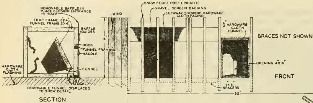
ENLARGED DETAIL OF FLASHING AND SCREEN FACINGS
