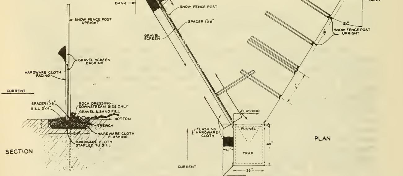
Figure 7.--Diagrams of Carp Creek sea lamprey weir.
