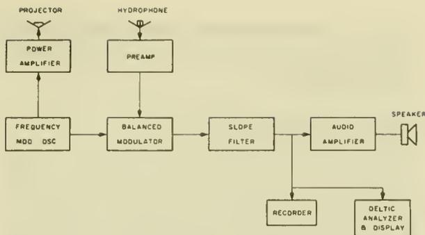
Figure 1.--Block diagram of fishery CTFM sonar system.
