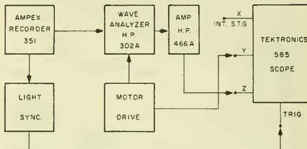
Figure 8.--Slow scan panoramic spectrum analysis block diagram.
