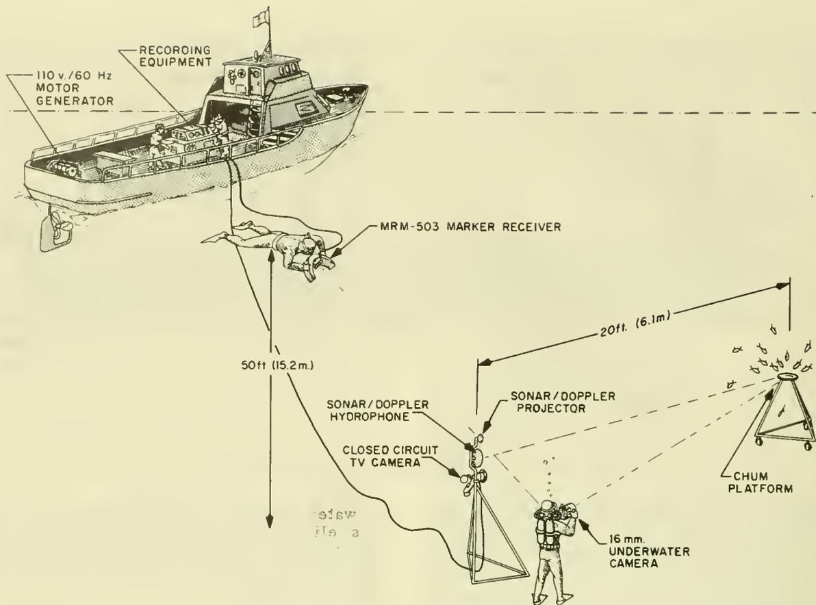
Figure 6.--Test arrangements at Catalina Island.
