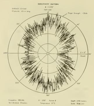
Figure 4.--Directivity pattern for a 60 cm. skipjack tuna rotated in the horizontal plane. The test frequency was 280 kHz. For this and foilowing figures the target range was 6 m., the temperature 21<sup>o</sup> C., and the test depths 3.9 m. Each ring represents a 10 db decrement from the outer - 20 db ring.
