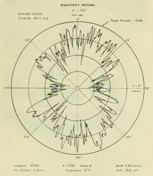
Figure 3.--Directivity pattern for a 60 cm. skipjack tuna rotated in the horizontal plane. The test frequency was 40 kHz. For this and foilowing figures the target range was 6 m., the temperature 21<sup>0</sup> C., and the test depth 3.9 m. Each ring represents a 10 db decrement from the outer -20 db ring.
