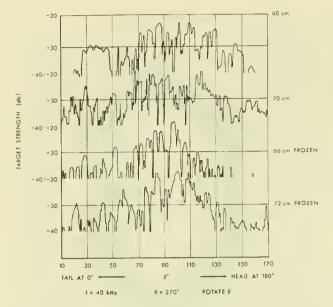
Figure 5.--Rectilinear plot of directivity patterns of 40 kHz (left side only) of four skipjack tuna. See text for explanation.
