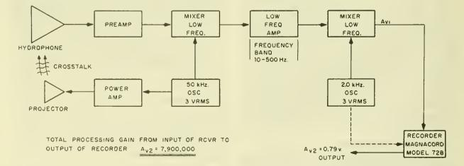
Figure 3.--Doppler sonar block diagram.
