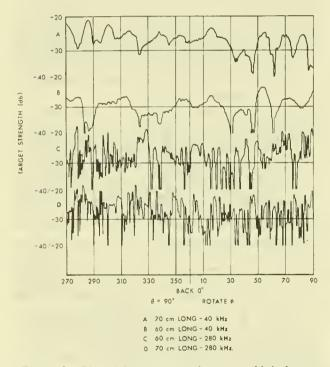
Figure 6.--Directivity patterns for two skipjack tuna suspended nose up, tall down and rotated about the long axis.
