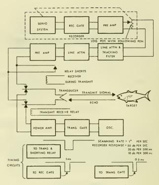
Figure 1.--Biock diagram of the test setup used to measure the target strengths of fish.
