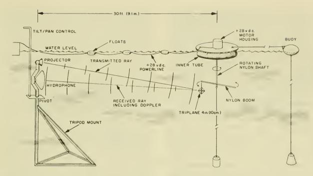
Figure 4.--Test arrangements at Lake Murray.
