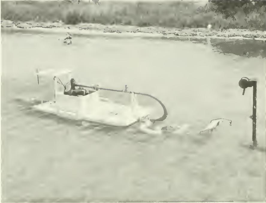
Figure 4.--The suction sampler in position for sampling in shallow water.
