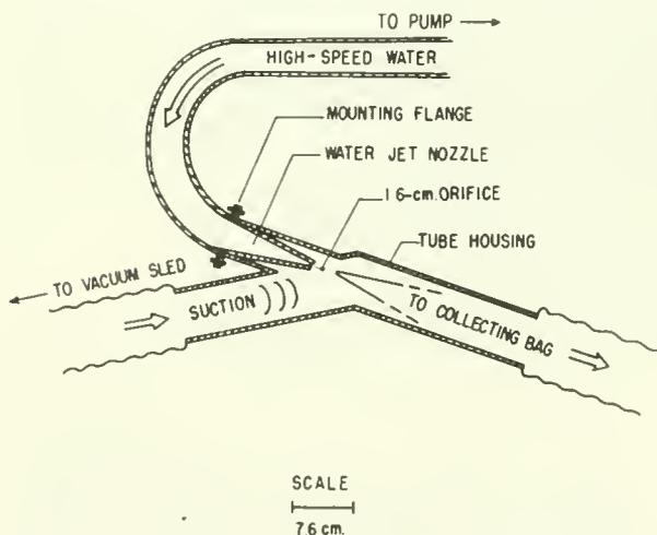
Figure 3.--Schematic drawing of the venturi tube.
