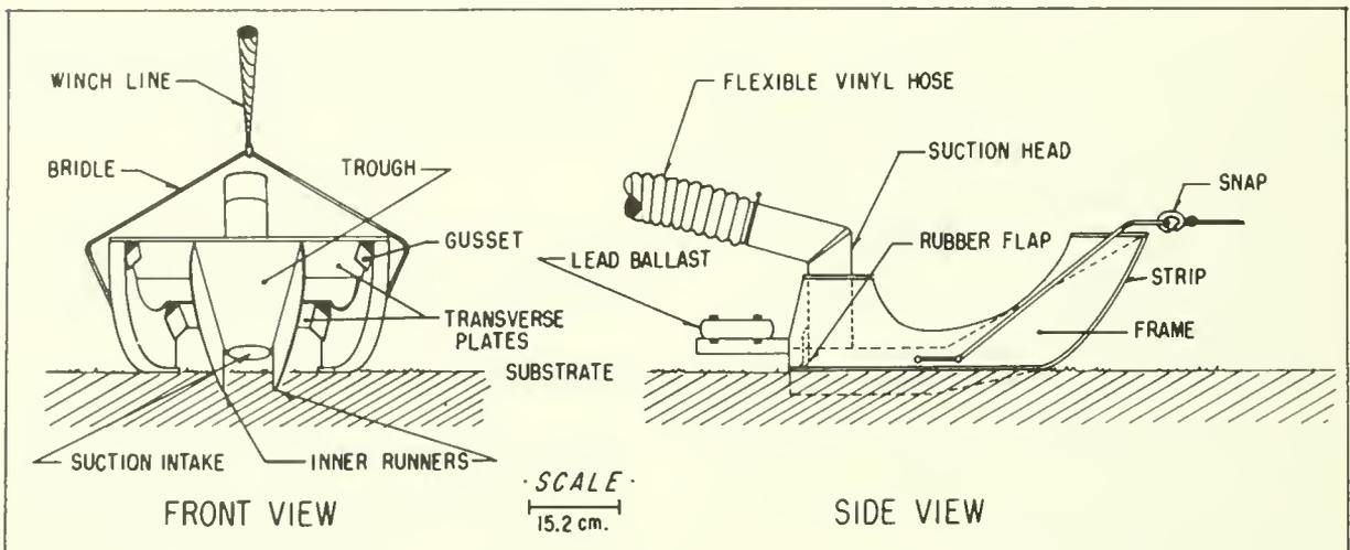
Figure 2.--Schematic drawings (front and side view) of the vacuum sled.
