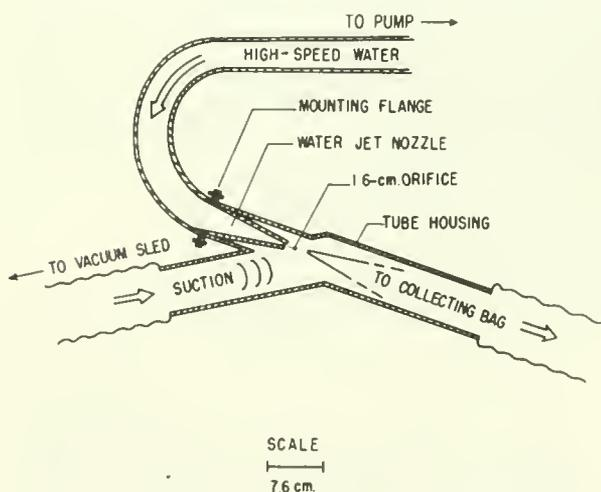
Figure 3.--Schematic drawing of the venturi tube.
