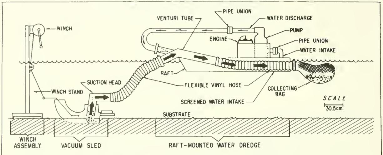
Figure 1.--Schematic drawing of the suction sampler.
