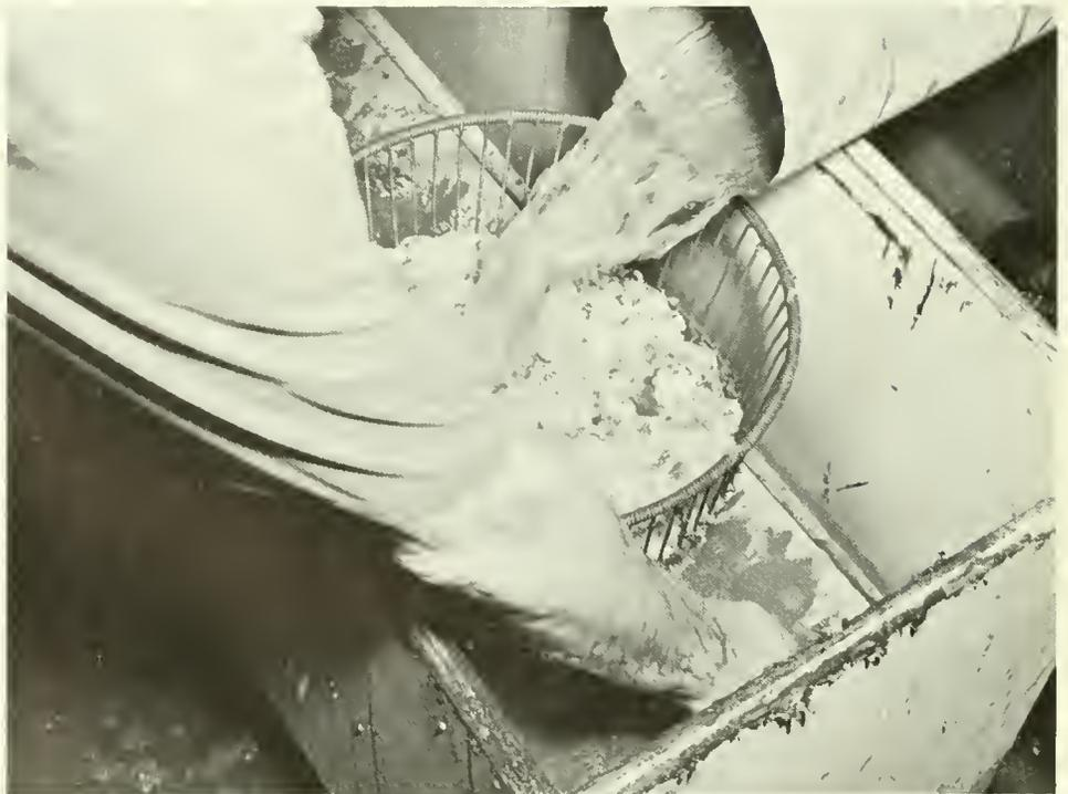
Figure 5.—View of scallop meats and viscera being collected into a wire-mesh basket from the discharge pipe from the vibrating screen.
