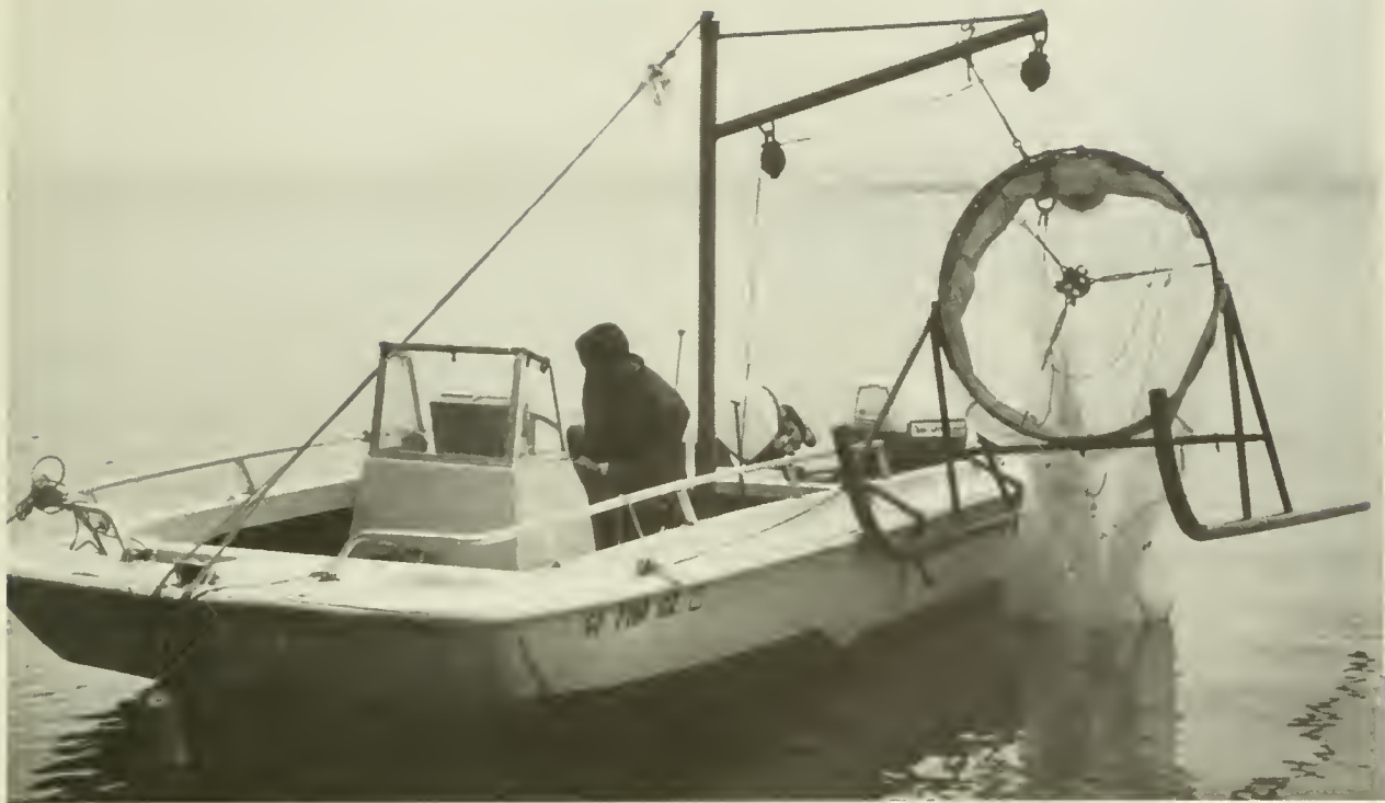
Figure 2. — Sampling boat showing macroplankton sampling apparatus.
