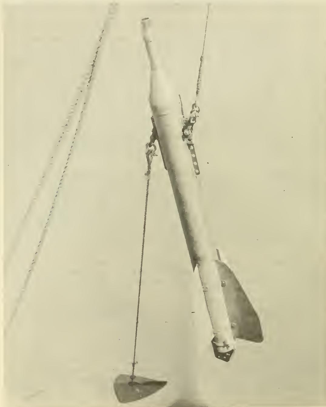
Figure 4. Model Gulf I-A high speed plankton sampler rigged in position for lowering.
