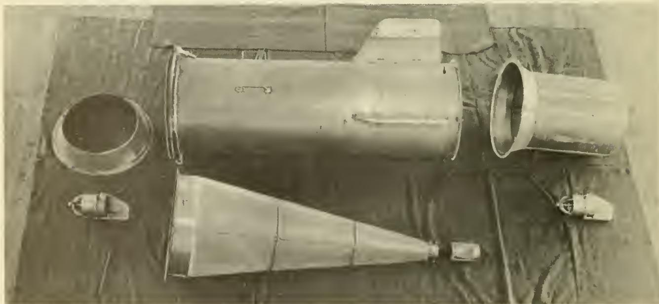
Figure 6. Exploded view of Model Gulf III plankton sampler.
