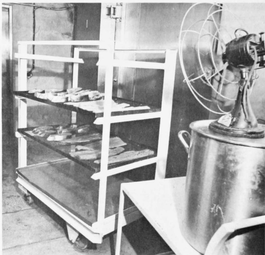
Figure 13.—Predrying by use of a fan.
