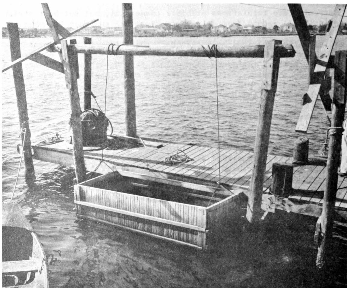
board, plywood, or planks. Water is pumped into the tank continuously for aeration and waste products are removed by the overflow. Most tanks of this type are shaded to keep the water cool and to prevent excessive plant growth. Both types are generally 4 by 4 by 8 feet. Pens of this size have a capacity of 25 to 30 quarts of live shrimp. Each dealer has two or three tanks; a few have as many as six.
