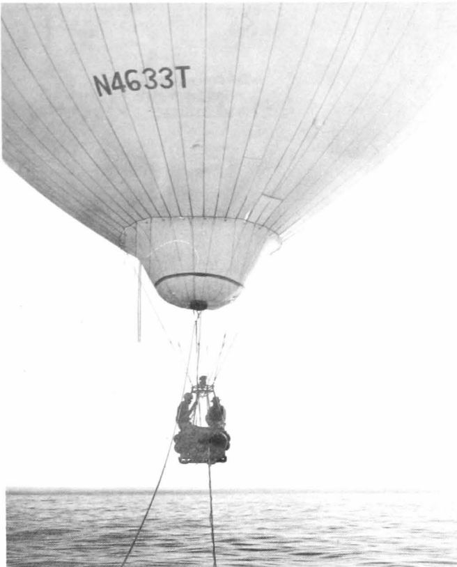
Figure 3.--Fishery scientists of the Tuna Resources Laboratory in cooperation with the Bureau's Oceanographic Instrumentation Unit and private industry conduct experiments with the use of tethered hot air balloons on fishing vessels to aid in detection of tuna and other pelagic fish schools.
