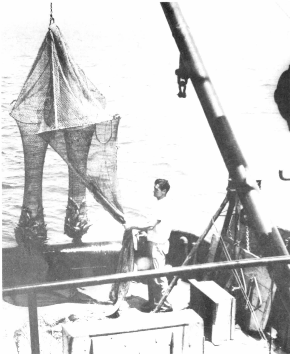
Experimental "trouser leg" cod end net on the R/V Kaho in the Great Lakes. Each "leg" is made of a different size mesh permitting simultaneous sampling to determine the most efficient gear for capture of desired size and species of fish.
