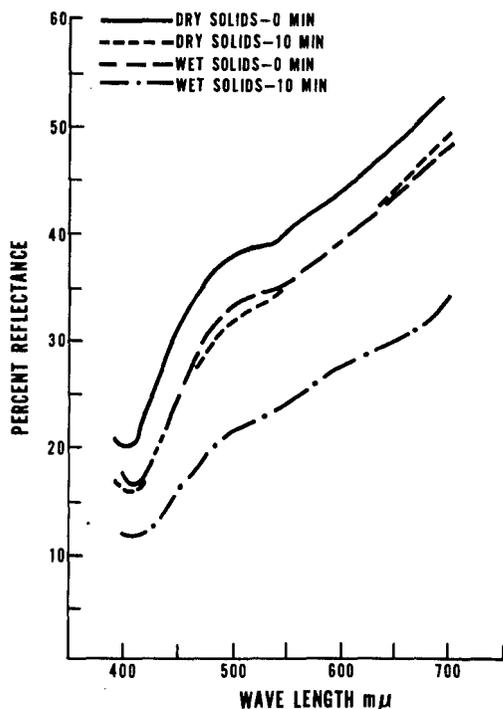
FIGURE 1.—Reflectance spectra of FPC's steam desolventized, as either dry solids or alcohol wet solids, at 2 to 3 psi for 0 or 10 min.
