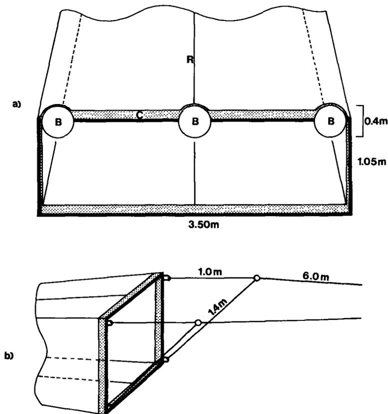
FIGURE 2a.—Front view of the neuston trawl; B = inflated 40 cm diameter spar buoys; C = cloth collar around mouth of net; R = polypropylene rib lines.
