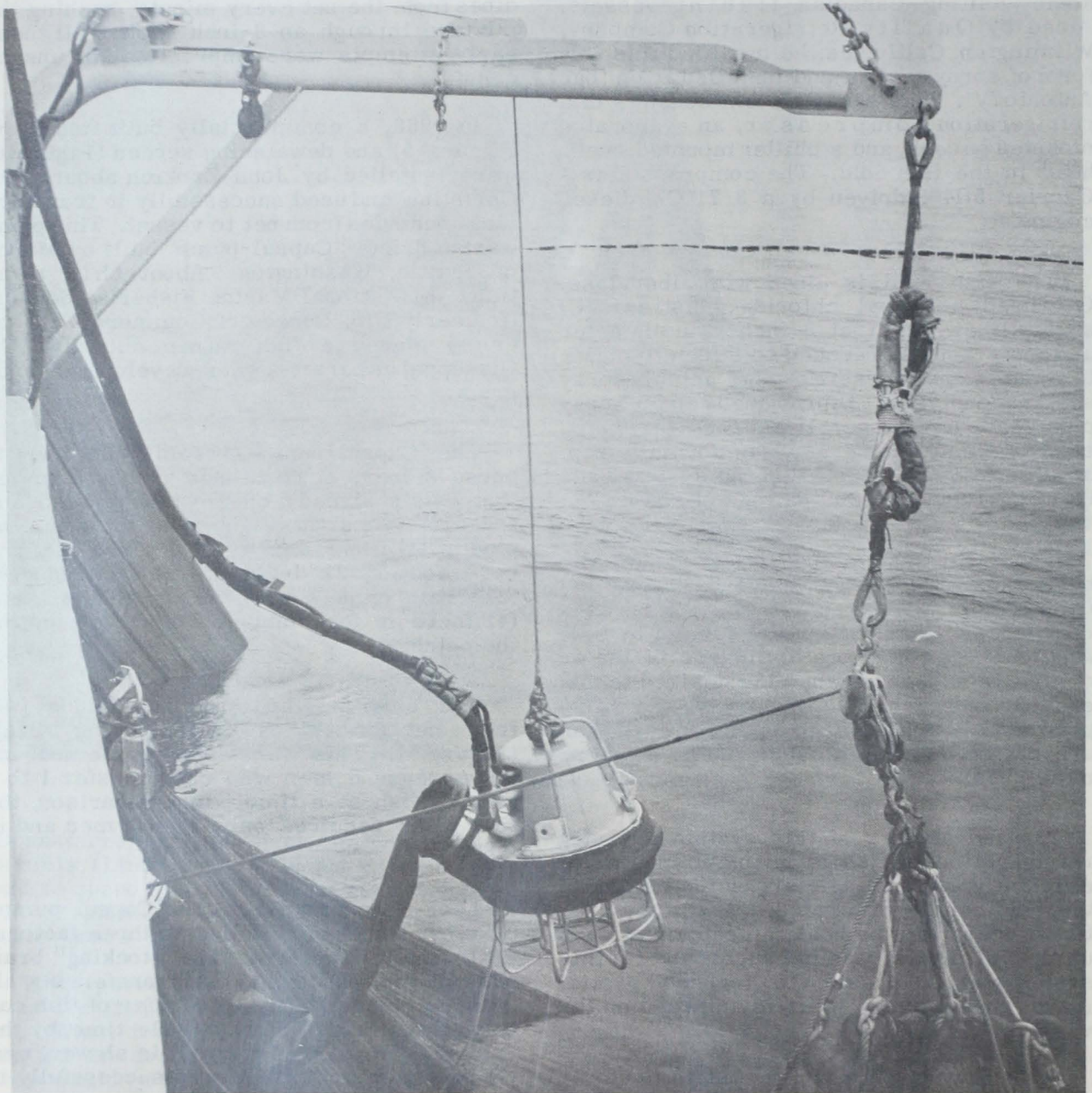
Fig. 5 - Capsul-pump attached to "Morgan" boom.
