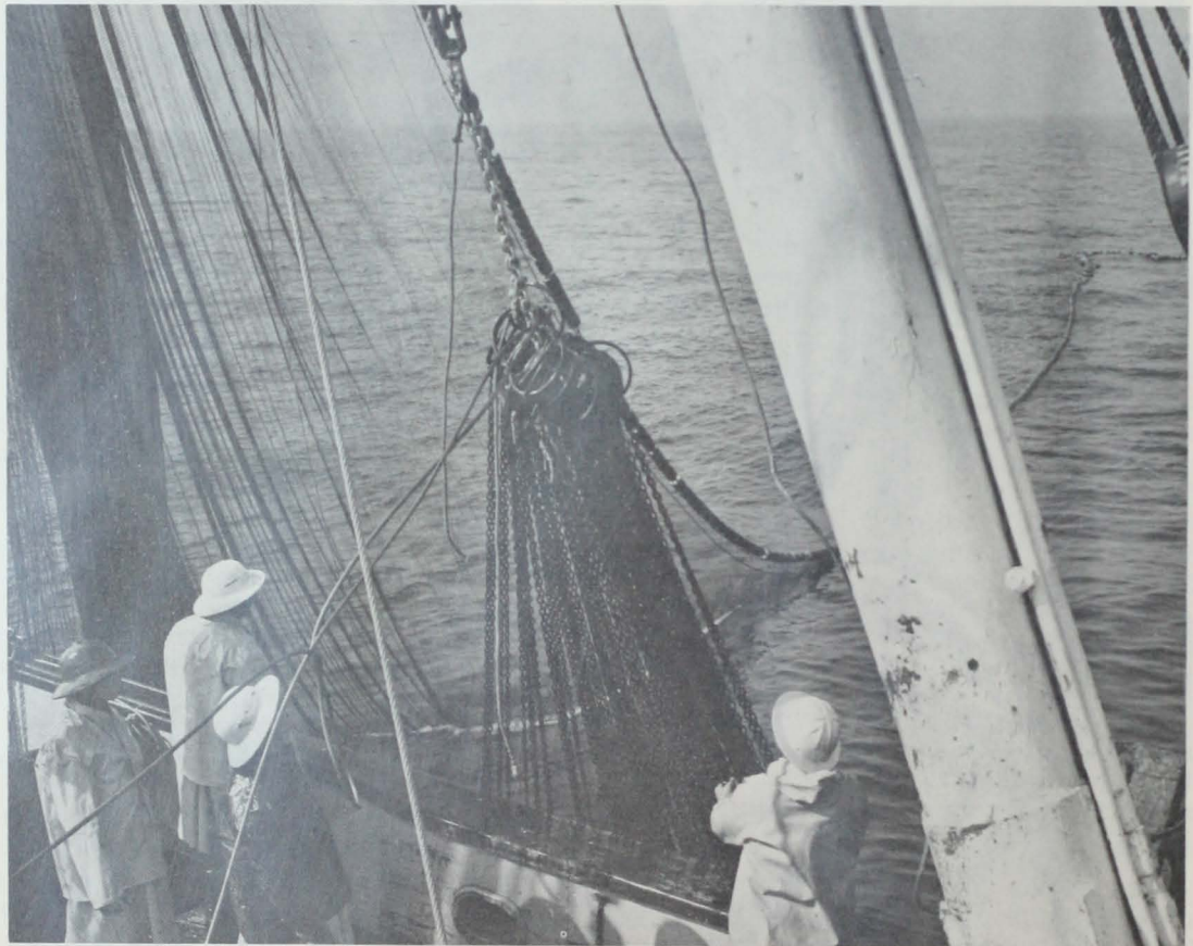
Fig. 14 - Purse rings being hoisted on deck.
