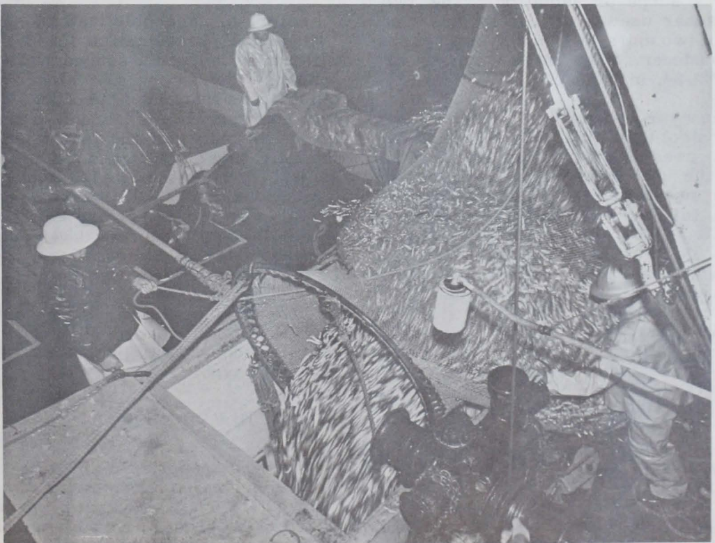
Fig. 7 - The stocking brail being used to transfer anchovies from the net to the boat.
