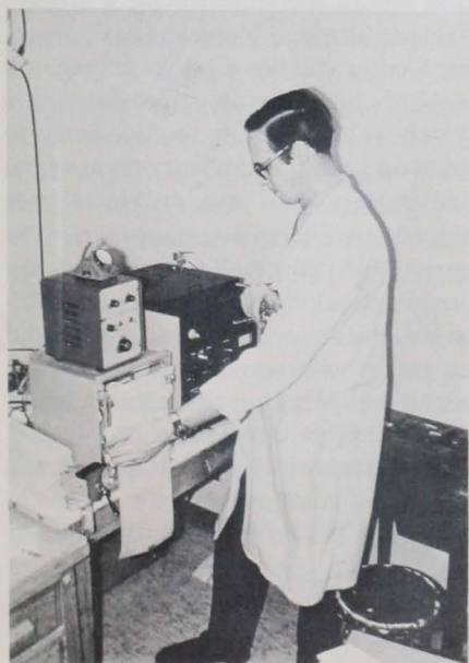
Analyzing of marine organisms by gas chromatography for amount of hydrocarbons.
