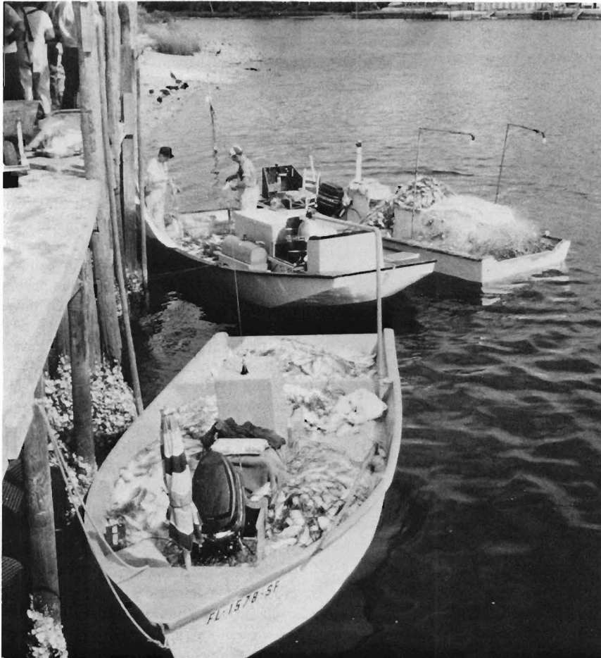
This type of boat is called a "well" boat and is powered by an inboard motor mounted through an opening in the hull.
