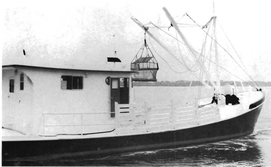
Figure 8.—Oyster vessel, the Conservationist , rigged with two booms and dredges (only one is shown) with bottom doors for emptying the oysters.
