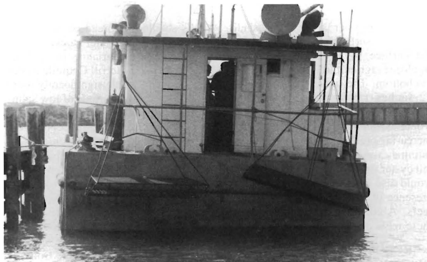
Figure 9.—Two machines for cleaning mud off oyster reefs attached to stern of motorized barge while at dock.
