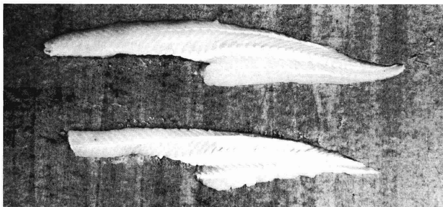
Figure 4.—Deep skinned ("defatted") fillets (above) or "regular" fillets (below) could be produced with a simple adjustment on the SFA-4 filleting and skinning machine.
