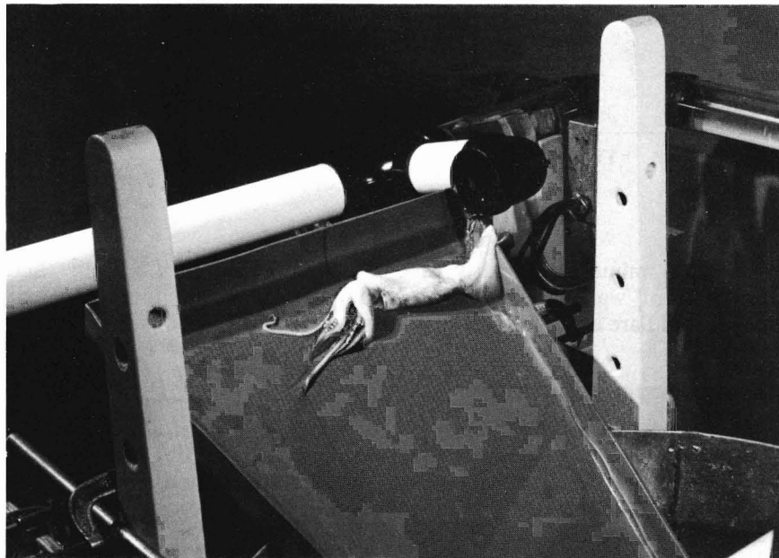
Figure 4.—Squid diverted from ducting and onto alignment slide.
