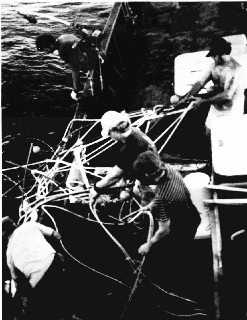
Figure 1.—An offbottom longline Kali pole tangle; clearing these are time consuming and may be dangerous to crew members.
