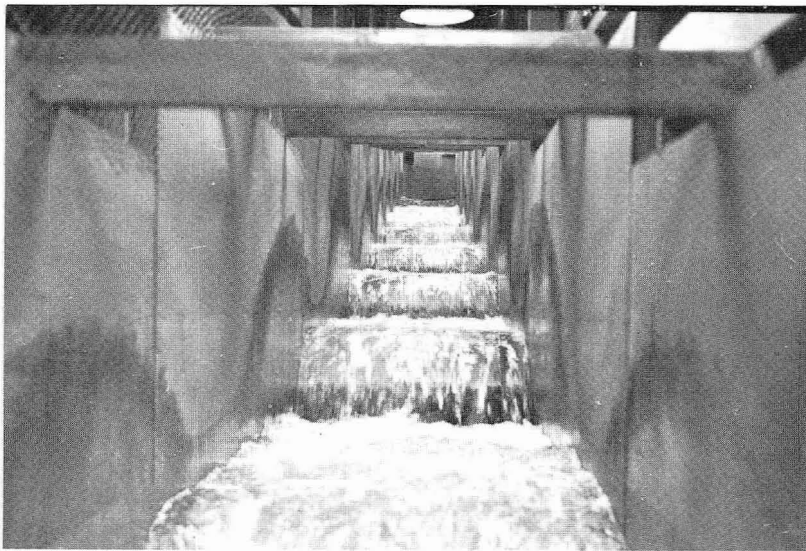
FIGURE 5.—Looking upstream from pool 53 in the 1-on-8-slope endless fishway.
