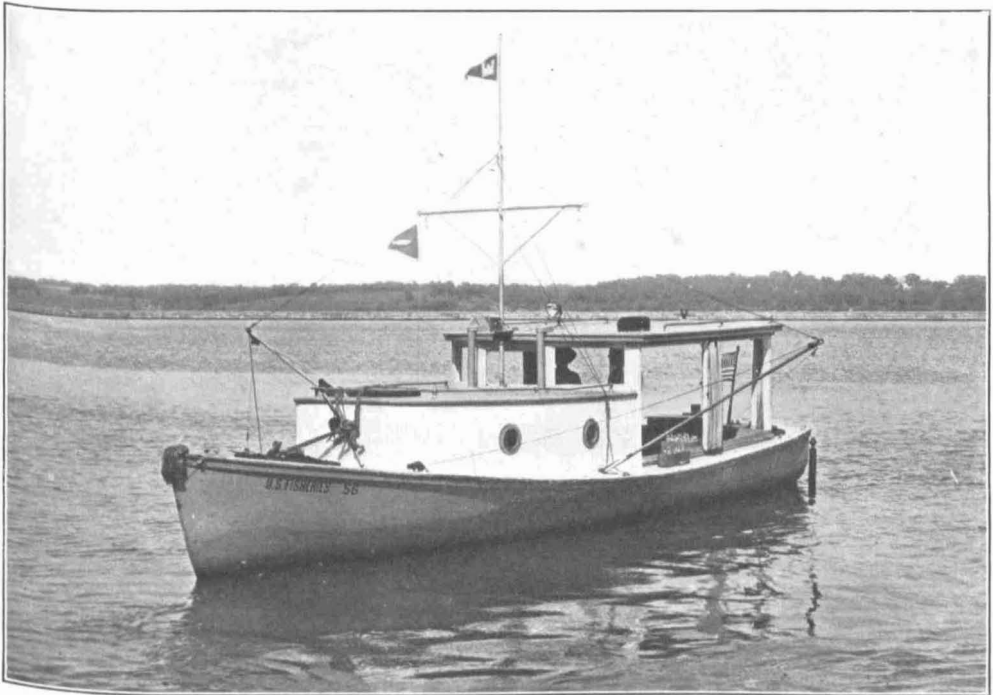
FIGURE 2.—U. S. Fisheries cruiser 56, equipped with sounding and sampling booms and field-laboratory apparatus. Two such cruisers were used on the larger rivers and streams.
