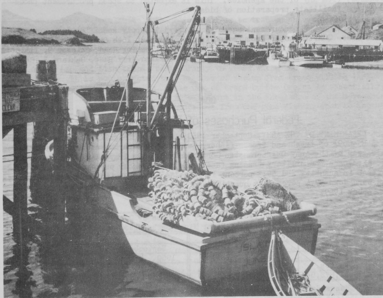
SALMON PURSE SEINER DOCKED AT KODIAK, ALASKA. PURSE SEINE NET IS STORED IN THE STERN OF THE BOAT. FISHING FLEET DOCKS CAN BE SEEN IN THE BACKGROUND.
