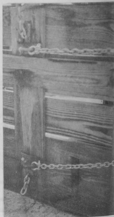
FIGURE 4 - METHOD OF ATTACHING PAD EYES AND CHAFING CHAIN TO OTTER BOARDS. (NOTE: TO OBTAIN MAXIMUM VERTICAL OPENING OF NET AND TO ASSURE ITS TENDING BOTTOM, PAD EYES SHOULD BE AS NEAR TOP AND BOTTOM OF BOARDS AS POSSIBLE.)
