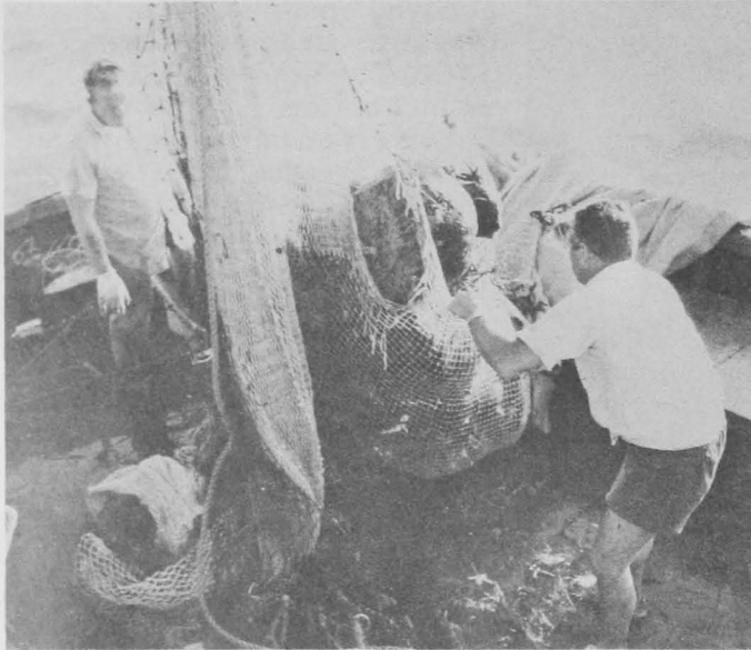
Fig. 9 - Overloading with loggerhead sponges is a major hazard to trawling in wide areas off southwest Florida. Catches of sponge are so heavy in some areas that nets cannot be hauled aboard.
