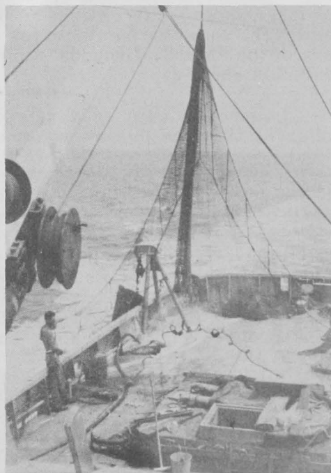
Fig. 8 - The 40-foot bottomless trawl developed for exploratory dragging on loggerhead-sponge bottom.
