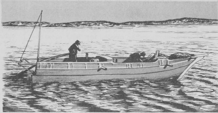
Typical small Japanese fishing boat used for set-net fishing in coastal waters.
