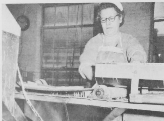
Pouring batter on fish sticks prior to breading in a leading Gloucester fishery products plant.
