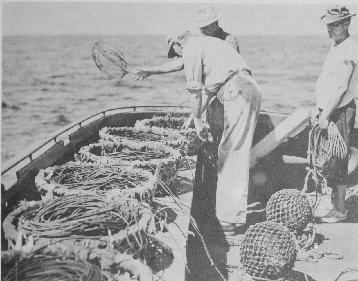
Fig. 3 - Setting the gear from the stern of the Oregon . Two men are used to keep the mainline and branch lines running clear. The third man stands by to heave the buoys.
