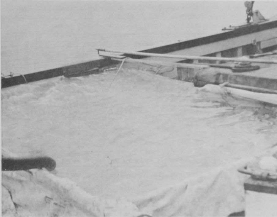
Fig. 2 - Receiving tank used to collect the fish which were pumped on board.
