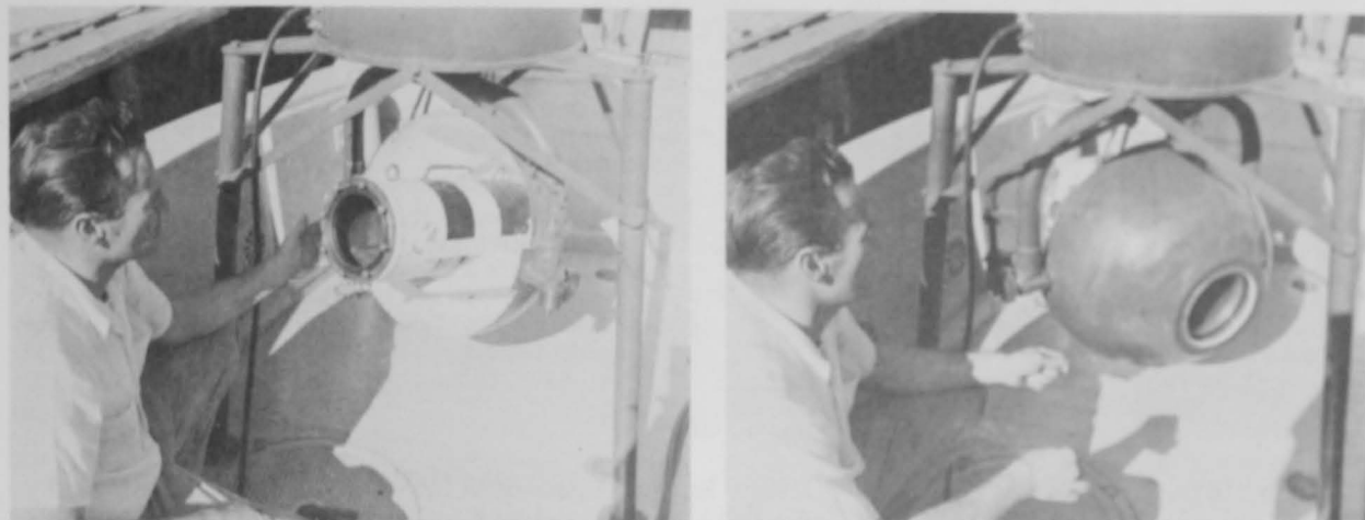
Fig. 8 - Experimental prototype tripod arrangement supporting remotely-controlled submersible power unit, with TV camera pressure cylinder mounted in a spherical free-flooding external housing capable of scanning 360^{\circ} in azimuth and 90^{\circ} in elevation. Left: rear view with half of spherical housing removed; right: front view.
