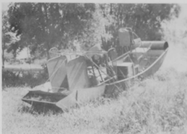
Fig. 3 - Airboat used in run-around gill-net operation showing extension on stern for net storage.
