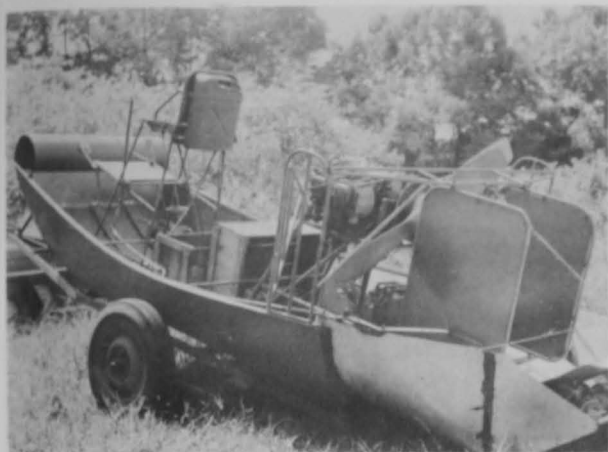
Fig. 2 - Airboat with gill net adaption mounted on trailer for transporting to various fishing grounds.
