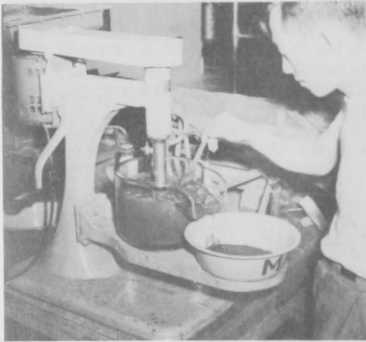
FIG. 1 - H. S. CHOI USING A FAGERGREN FLOTATION CELL TO INVESTIGATE THE USE OF FISH OIL FATTY ACIDS IN ORE CONCENTRATION. THE HEAVY GLASS CELL CONTAINS AN AQUEOUS PULP OF FINELY-GROUND IRON ORE. FATTY ACIDS SELECTIVELY COAT THE IRON OXIDE MINERAL PARTICLES, MAKING THEM HYDROPHOBIC. MECHANICAL STIRRING OF THE PULP AND SIMULTANEOUS ADMISSION OF AIR PERMITS THE COATED IRON OXIDE PARTICLES TO BECOME ATTACHED TO AIR BUBBLES, WHICH RISE TO THE SURFACE AND ARE SCRAPPED INTO THE PAN IN FRONT OF THE OPERATOR, THUS PRODUCING AN IRON-RICH CONCENTRATE. THE SILICEOUS GANGUE MINERALS, BEING HYDROPHILIC, REMAIN IN THE PULP AND DO NOT CONTAMINATE THE CONCENTRATE, THUS PRODUCING A TAILING.
