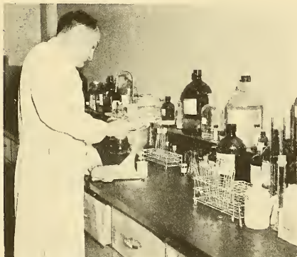
FIG. 1 - EMULSIFYING MENHADEN OIL FOR OXIDATION STUDIES AT THE FOOD TECHNOLOGY LABORATORY, UNIVERSITY OF CALIFORNIA, DAVIS, WHERE A PORTION OF THE PROGRAM ON OXIDATIVE DETERIORATION OF FISHERY PRODUCTS IS BEING CARRIED OUT.
