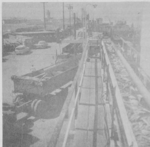
FIG. 5 - A TYPICAL CONVEYOR OR FLUME USED TO CARRY FISH FROM TRUCKS TO CANNERY.
