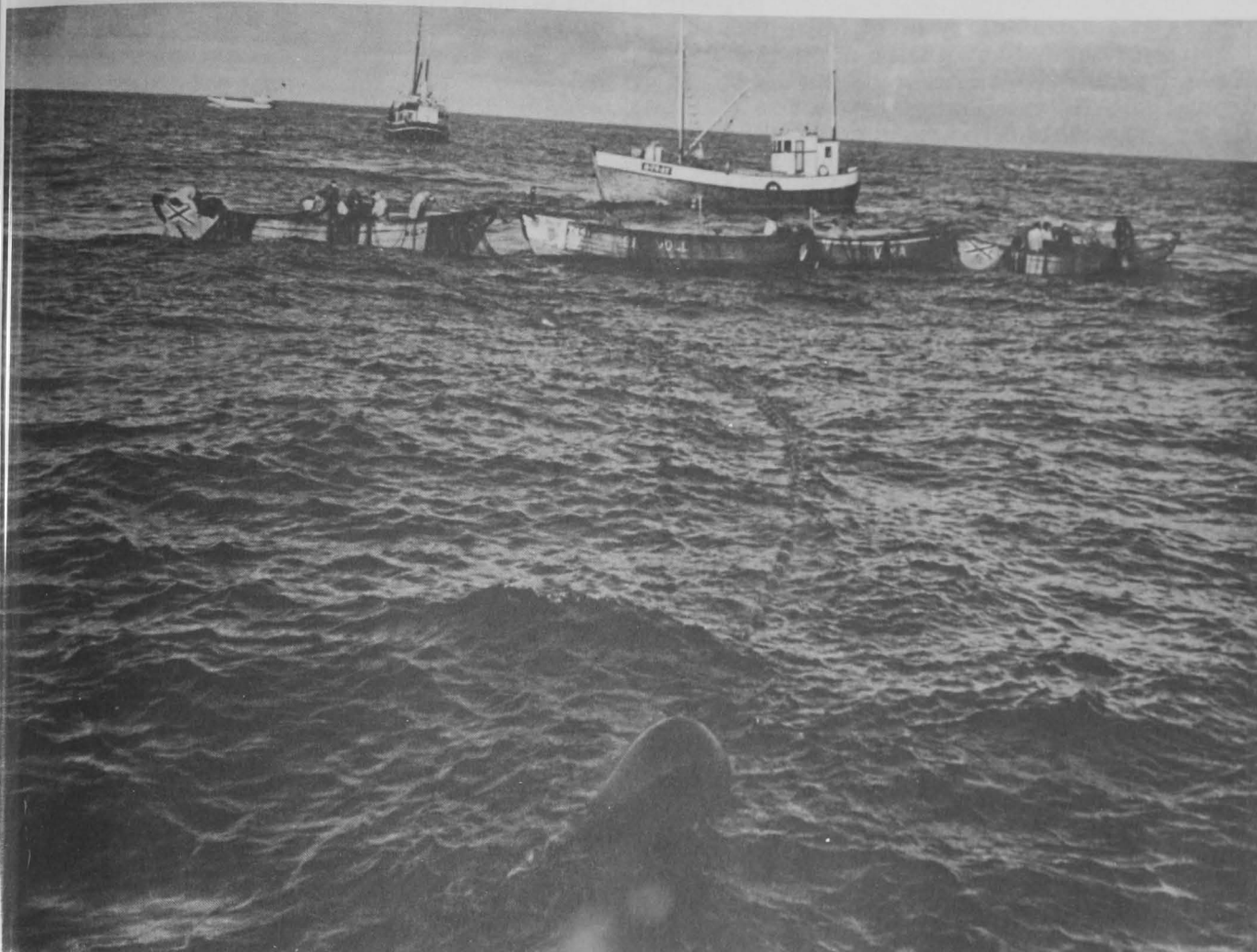
A large purse seine has been set around a submerged school of herring. The seine has been pursed and the net is being dried into the mechanized purse seine dories for confining the fish more closely in the bag of the net.
