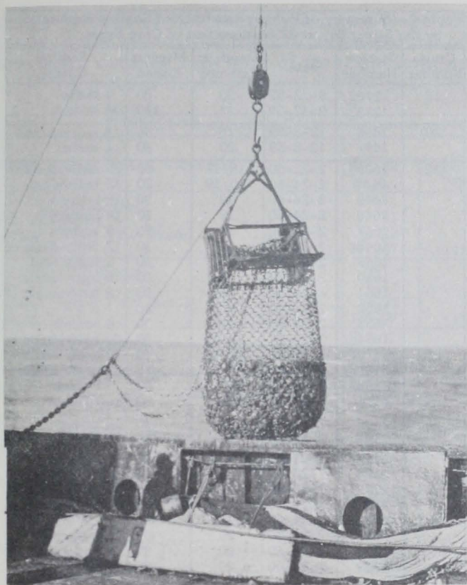
Fig. 3 - A 14-tooth Fall River clam dredge coming aboard the Silver Bay with approximately 4 bushels of hard clams.
