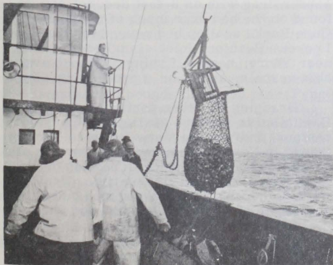
Fig. 4 - A 14-tooth Fall River clam dredge coming aboard the Silver Bay with approximately 6 bushels of hard clams.
