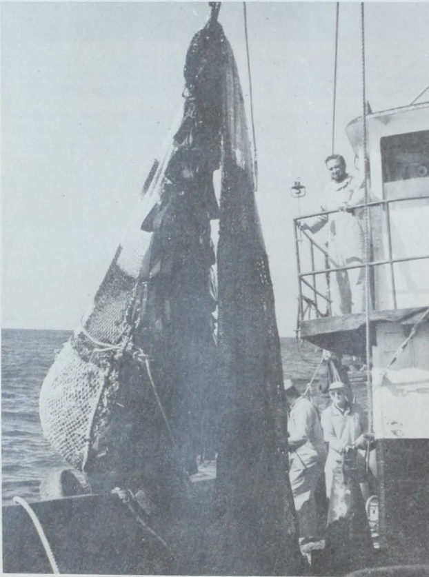
Fig. 7 - A roller-rigged nylon fish trawl coming aboard the Silver Bay with approximately 2,000 pounds of industrial fish.
