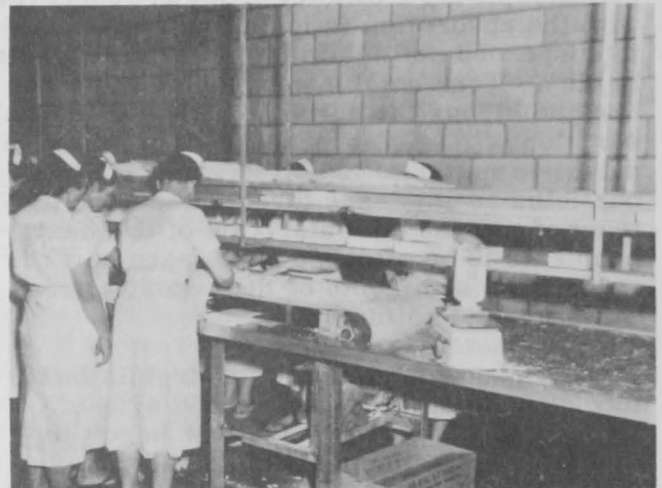
Breaded shrimp is packed in cartons prior to freezing in a shrimp-breeding plant located in Brunswick, Ga. Packed boxes on center belt conveyor are carried to weigher.
