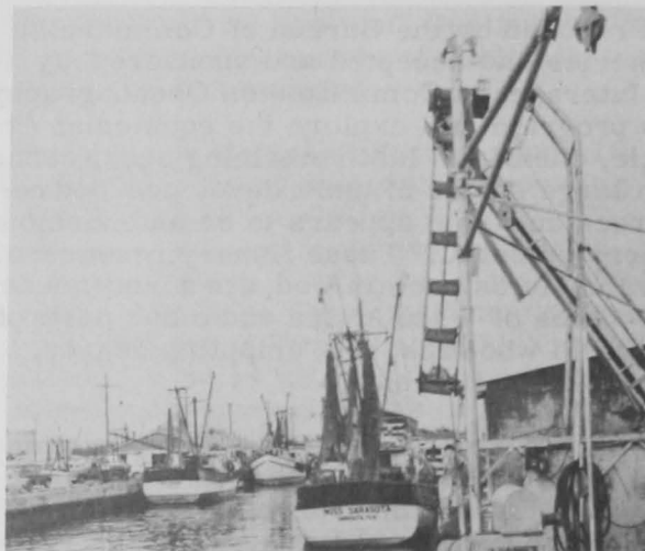
Bucket unloader used for unloading shrimp from trawlers, Tampa, Fla.
