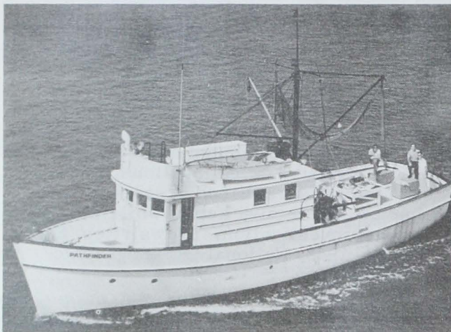
Research vessel, Pathfinder , traverses area monthly recording temperatures and salinity data every three miles.
