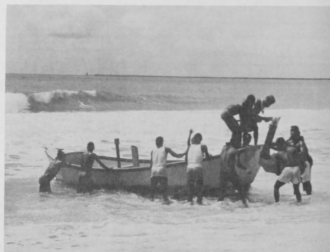
In 1956, a 20-foot aluminum surf boat was designed and built for the Federal Fisheries Department of Nigeria by a British shipyard. It was an experimental vessel designed for ring-net fishing. This shows the first trials of the boat and the rudder being placed in position.
