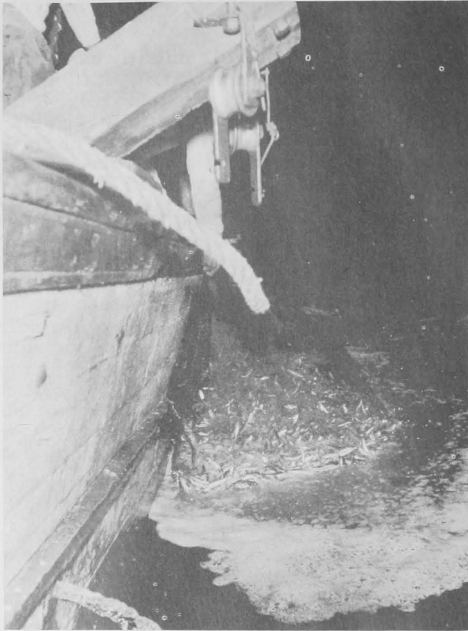
Fig. 3 - In Tunisia a vessel fishing at night is equipped with electric surface lamps for attracting fish. Here a net-load of fish is being hauled aboard.
