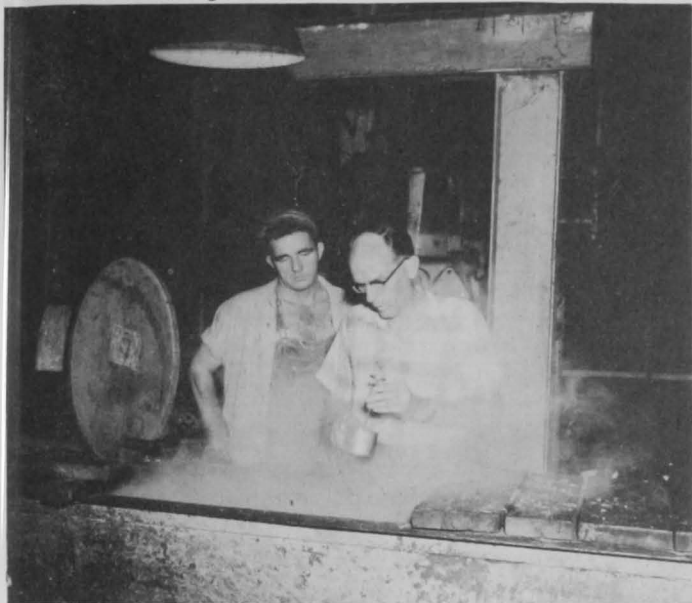
Chemist is determining the temperature of press cake being discharged from the screw press in a Moss Point, Miss., industrial fishery products plant.
