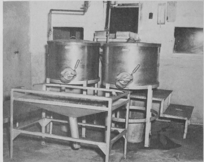
Fig. 20 - Shown here is another high-mounted blower installation. These two medium-size tanks would handle oysters from 20 to 30 shuckers. Small plants employing up to 15 shuckers often have only one blower.
