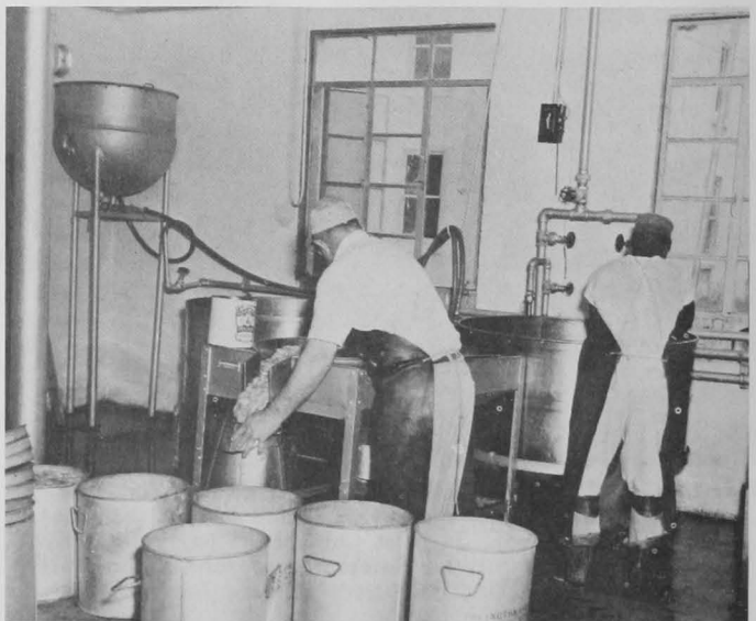
Fig. 22 - One worker empties the tank while the "skimmer man" fills a 5-gallon measure. Oysters are held in the 5-gallon cans (foreground) until they can be packed into smaller units. Often this repacking will be done in a large central plant.
