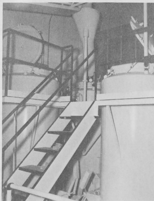
Fig. 40 - One oyster cannery uses vertical autoclaves, filled from overhead conveyors with the raw shellstock, for cooking the oysters.
