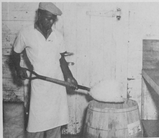
Fig. 27 - Cans are thoroughly iced before being shipped. A number of plants now have their own flake-ice machines to assure a plentiful supply.
