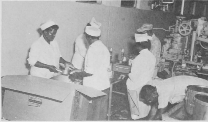
Fig. 29 - Some oysters are frozen in small cans. In this method of packing, the weight of oysters in each can must be checked on the scales because cans cannot be completely filled, owing to the expansion of the product when frozen.
