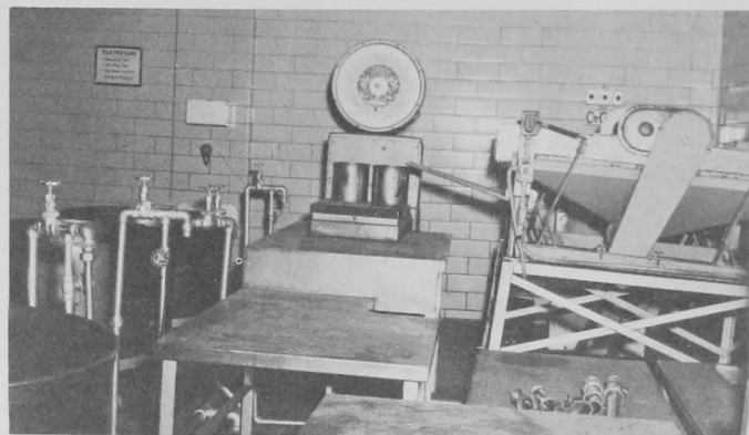
Fig. 24 - This plant uses a power-driven vibrating delivery skimmer and weighs the drained oysters instead of measuring the volume.
