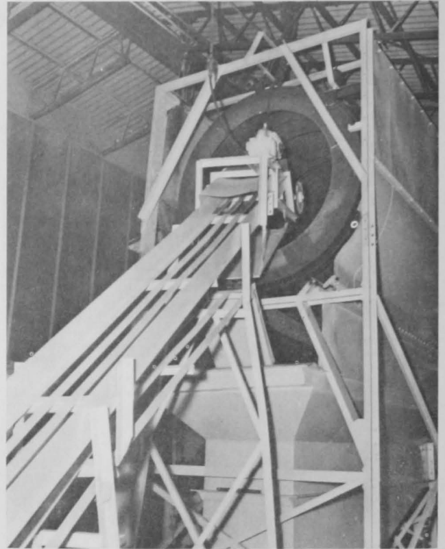
Fig. 44 - Almost all canneries now have replaced hand labor with some modification of the mechanical shucker shown here. The steamed shellstock is tumbled in this rotating cylinder. The meats are shaken loose and fall through the slots into the tank below.
