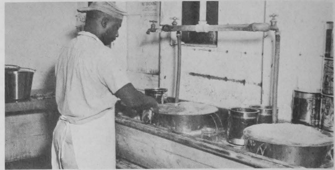
Fig. 18 - In many Gulf Coast plants, oysters are washed, 1 or 2 gallons at a time, in a dishpan with flowing water. The washing period is usually about 3 to 4 minutes.
