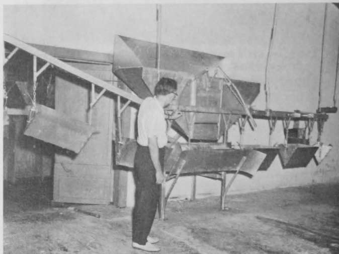
Fig. 10 - This filling hopper and the V-shaped "cars," which ride an endless track, make a conveyor system that was especially designed for maximum flexibility in moving the shellstock to the shuckers.
