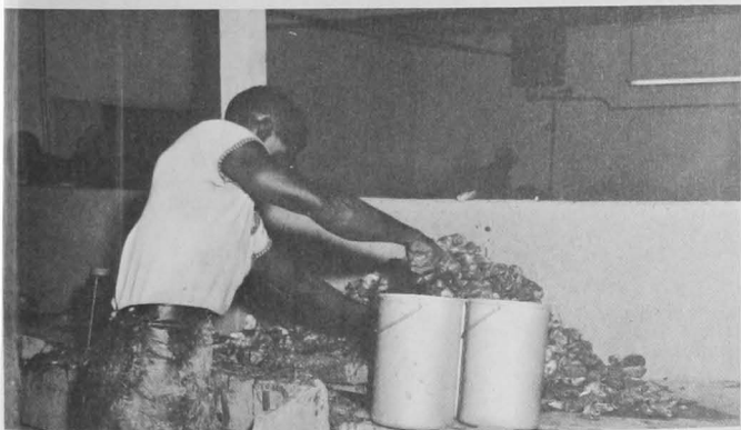
Fig. 15 - Another stroke of the knife cuts the muscle loose from the bottom shell, and the shucker then flips the meat into the shucking pot. In most Chesapeake Bay plants, each shucker has 2 or 3 pots for different sizes, and he does all grading for size.
