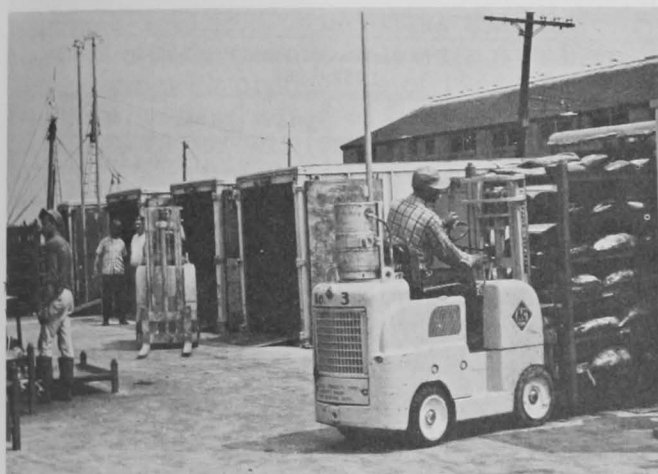
Fig. 5 - Forklift truck loading six-foot high pallets or racks into truck for transport to freezer.
