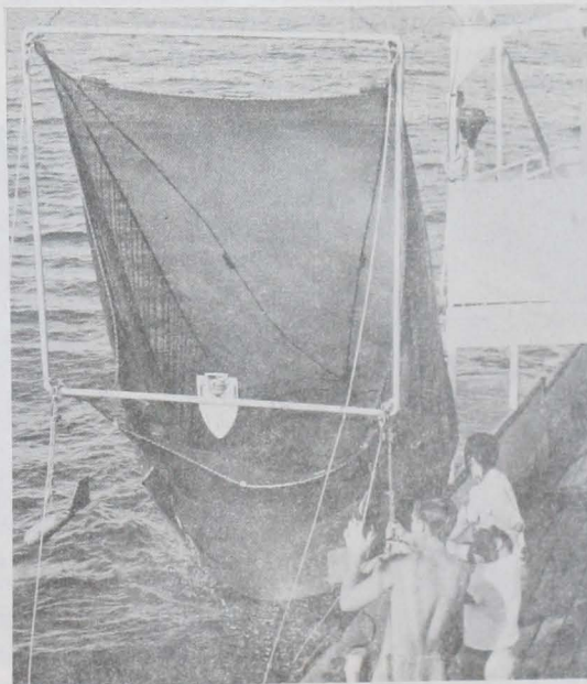
Fig. 2 - A plankton net with 2-meter opening to the side (designed by a U. S. Bureau of Commercial Fisheries biologist).
